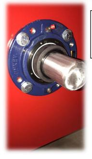
A 2 ½" Hardened steel shaft that is runs on the best quality solid steel TIMKEN bearings made USA.
