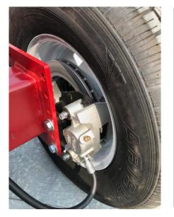
Brake system activated by hydraulic hand pump integrated in the machine with pressure gauge for easy set up to achieve best results when compacting the bag.
