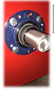
A 2 ½" Hardened steel shaft that is runs on the best quality solid steel TIMKEN bearings made USA.
