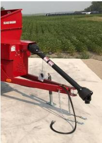
Heavy duty 540 PTO drive with shear pin protection.
