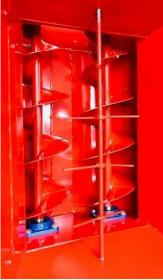
Our double screw system performs uniform compaction in the bag.
